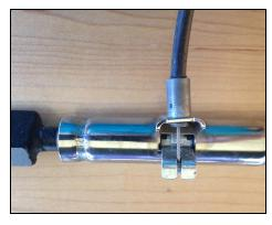
Note that the headpiece is designed to be used without the Remote (the remote just makes it more convenient). Until the new part arrives, you can remove the broken piece and manually operate the headpiece by squeezing the two metal tabs together with your fingers to activate the flexion / extension.
