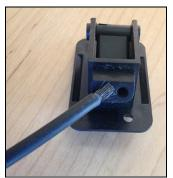
The primary reason that the Remote Control malfunctions is because the cable has frayed. **(photo)**
